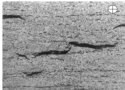
HIC step cracks
